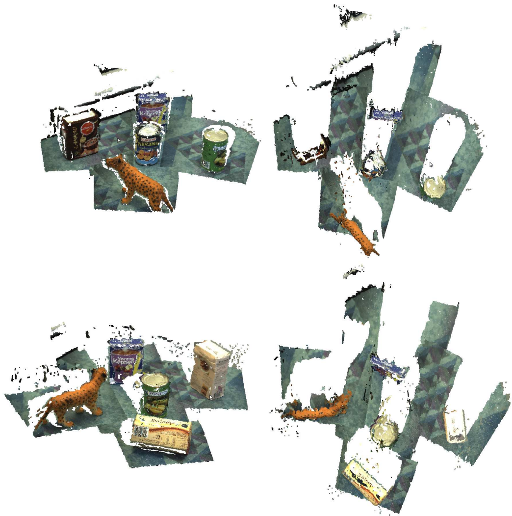
Fig. 7. Two examples (one each row) for a point cloud representing a whole scene merged from different view points. Left Column: View from the side. Right Column: View from the top.
