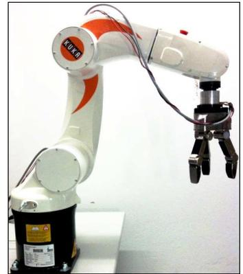
(b) Kuka Arm and Schunk Hand.
