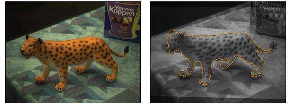
(a) Left Foveal Camera. (b) Segmentation on Overlaid Fixated Rectified Left and Right Images.
